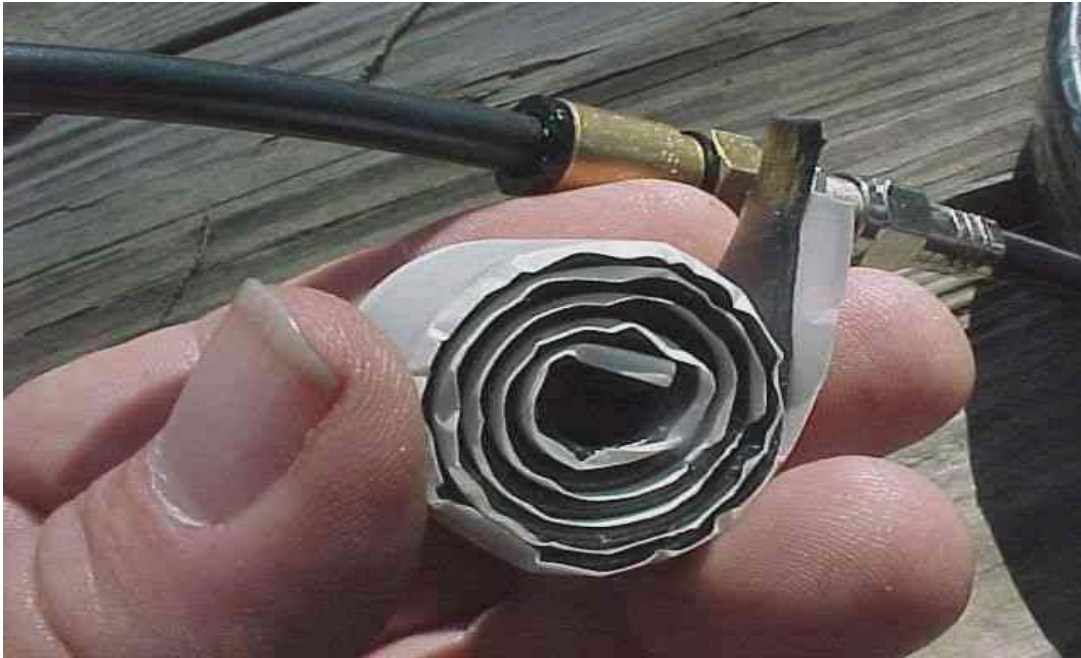
This picture show: A small roll of Coax-Seal. It is a putty like material in tape form. The white waxed paper keeps it from sticking to its self.
